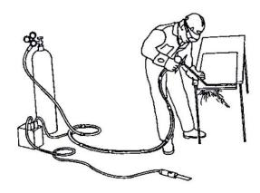
The **Prime Cut** system can also be connected to a welding machine. The welding machine is used only for igniton of the system. The torch is connected at the positive terminal of the machine and the copper striker plate is connected at the negative terminal. The welding machine is set at low amperage (50 amps.) by using an AC or DC current (DC preferred).
